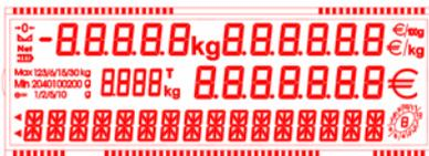
Backlit alphanumeric display with high contrast on both sides of buyer and seller with a 7 segment line for Weight, Price and Amount and 16 digits and 14 segments alphanumeric line for product description and menu options.
